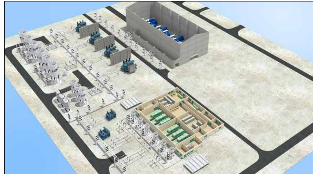
Figure 3: 3D model of an upcoming STATCOM station in India (Courtesy: Montnets Rongxin Technology Group Co., Ltd)
